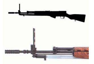
Type: Self-loading rifle Cartridge: 7.62x39mm Distinguishing features: Ribbed grenade launcher at muzzle; folding grenade sight
