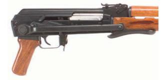
Type: Assault rifle Cartridge: 7.62x39mm Distinguishing features: Under-folding stock with
