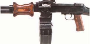
Type: Light machine gun Cartridge: 7.62x39mm Distinguishing features: Small, bulbous hand guard; drum-shaped belt magazine
